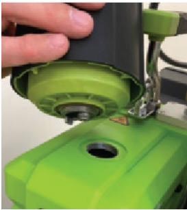
FIGURE 7: Demister removed, showing oil opening
